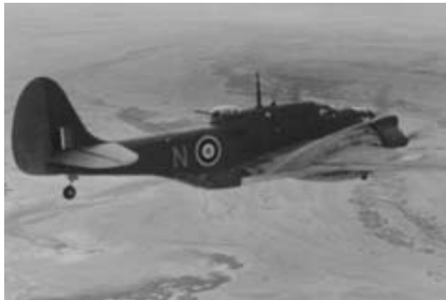
Aircraft 'N' goes out on sortie. This is a Mk IV and has the heavier turret with 0.5in guns.
