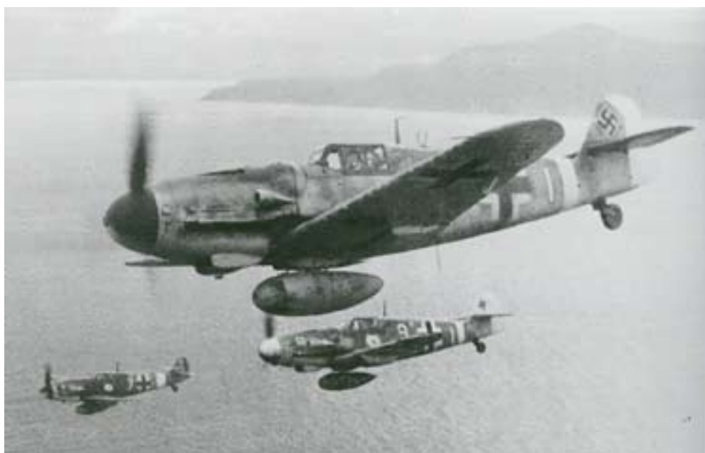
More formidable and responsible for a number of 454 losses was the Me-109F's of JG 27. The fighters were a proven design and deadly with one 20mm cannon and two 7.9mm machine guns in the nose.
