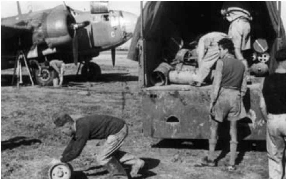
Armourers loading bombs prior to a sortie. The bombs were roughly handled, safe until fuses were installed. Gray Collection
